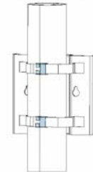
Figure 19 Installing the installation plate to the pole
