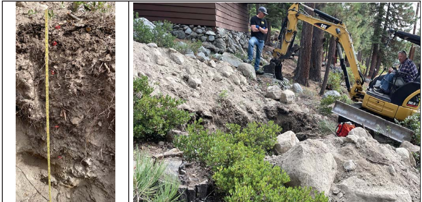
Photo A – View of soil profile showing bottom depth of 60+ inches. Fine and medium root penetration in substratum. No indication of seasonal water table. HSG-B.
