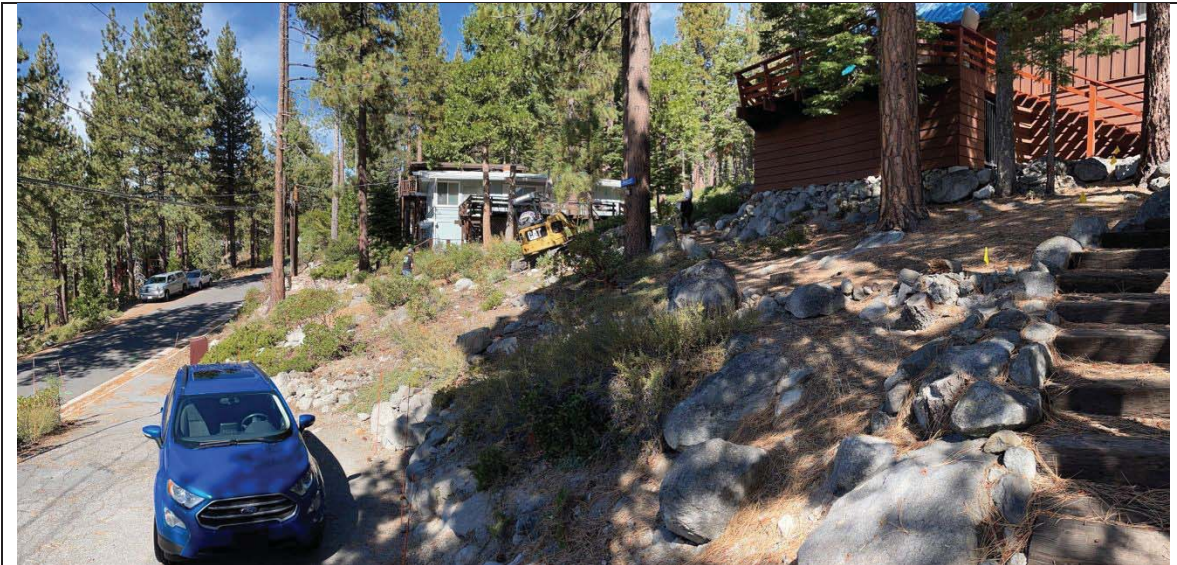
Photo 5 – View to north at driveway (left) and stairs to residence (right). The slopes immediately above and below driveway are artificially steepened. Natural slopes in this area are 33% (apparent on parcel immediately to south), which qualifies such land as Class 1A. The soil pit location (center, background) was undisturbed, except for fire protection vegetation thinning.
