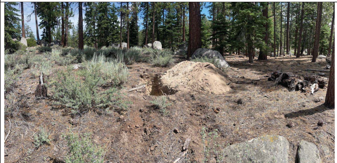
Photo 4 – View to northeast at Soil pit no. 3, located in the north-center of the subject parcel. This soil qualifies as Class 6, as per Land-Capability Classification of the Lake Tahoe Basin, California-Nevada (Bailey, 1974). This location has 4 to 10% slopes that dip to the south. The upland forest is dominated by Jeffrey pine and lesser amounts of white fir and incense cedar. The understory vegetation consists of sagebrush, bitterbrush, greenleaf manzanita, and scattered grasses/forbs. While variable, the vegetated ground cover in this vicinity is 30 to 40% and duff cover is 60 to 70%.
