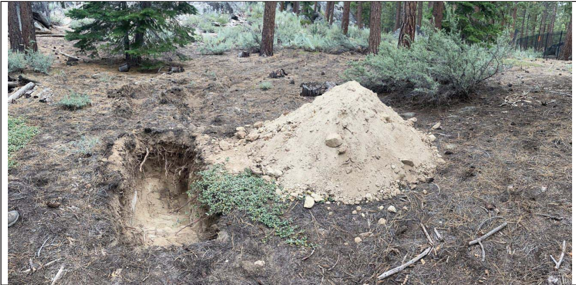
Photo 7 – View to northeast at Soil pit no. 4, located near the south corner of the property. Slopes in this area are 8 to 12%, dipping to the southwest. While the duff layer is only 1 inch thick here, the soils are sufficiently sandy and have granular to subangular blocky structure that effectively transmits rain and snowmelt through the profile. Such conditions are consistent with Hydrologic Soil Group A (no subsurface water and no limitations for root penetration). Soil erosion within parcel is very low and regeneration after disturbance is relatively quick.
