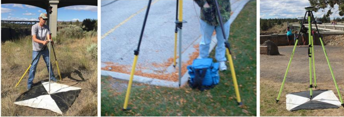
Figure 4. Surveying ground control points (GCPs) for UAS SfM photogrammetry using GNSS and total station.
