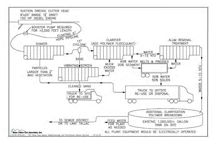
Figure 2-11 Dredge Dewatering Schematic Drawing.
