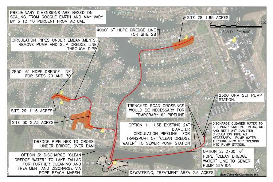
Figure 2-10 Preliminary Layout of Suction Dredging Operations.
