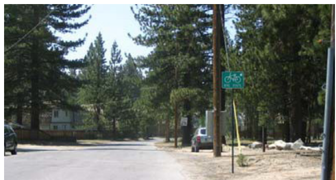
Bike Route/Shared Signed Roadway
