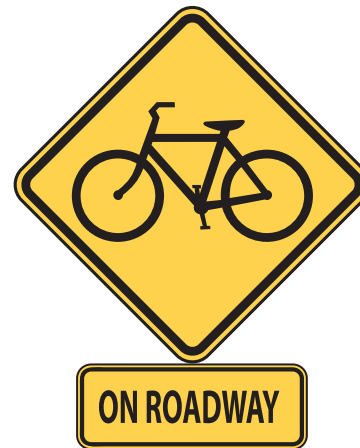
W11-1 with custom “ON ROADWAY” legend plaque. Under MUTCD 2C.03 P04, a state or local road agency is permitted to use word messages on warning signs other than those shown in the MUTCD.
