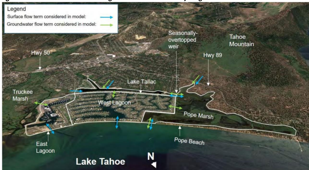
Figure 3. Schematic of the Water Budget Model of the Tahoe Keys Lagoons
