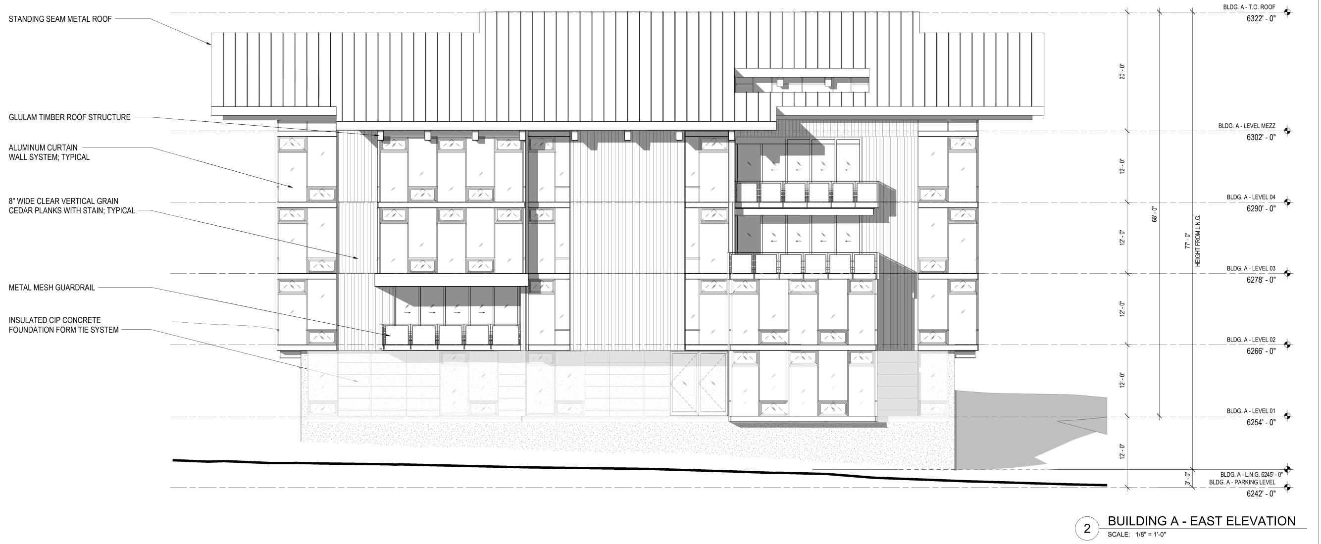
(02) (09) 9' - 6" 11' - 8 3/4" 23' - 10" 11' - 8 3/4" 17' - 0" 23' - 10" 17' - 0" 20' - 11 1/8" 45' - 0 3/4" GLULAM TIMBER BLDG. A - T.O. ROOF 6322' - 0" ROOF STRUCTURE STANDING SEAM METAL ROOF BLDG. A - LEVEL MEZZ
