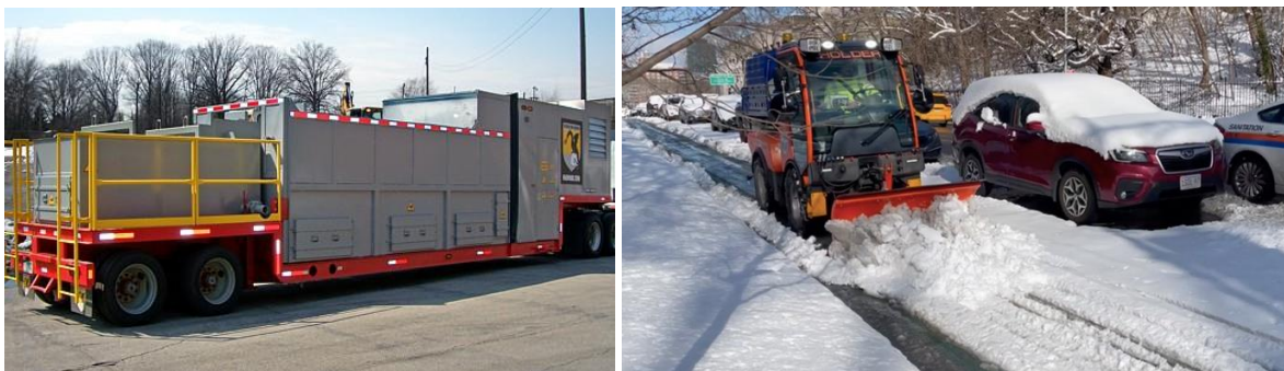
Left: Snow Dragon snow melting device. Right: Snowplow designed specifically for sidewalks and bicycle facilities (image: streetsblog.org)
