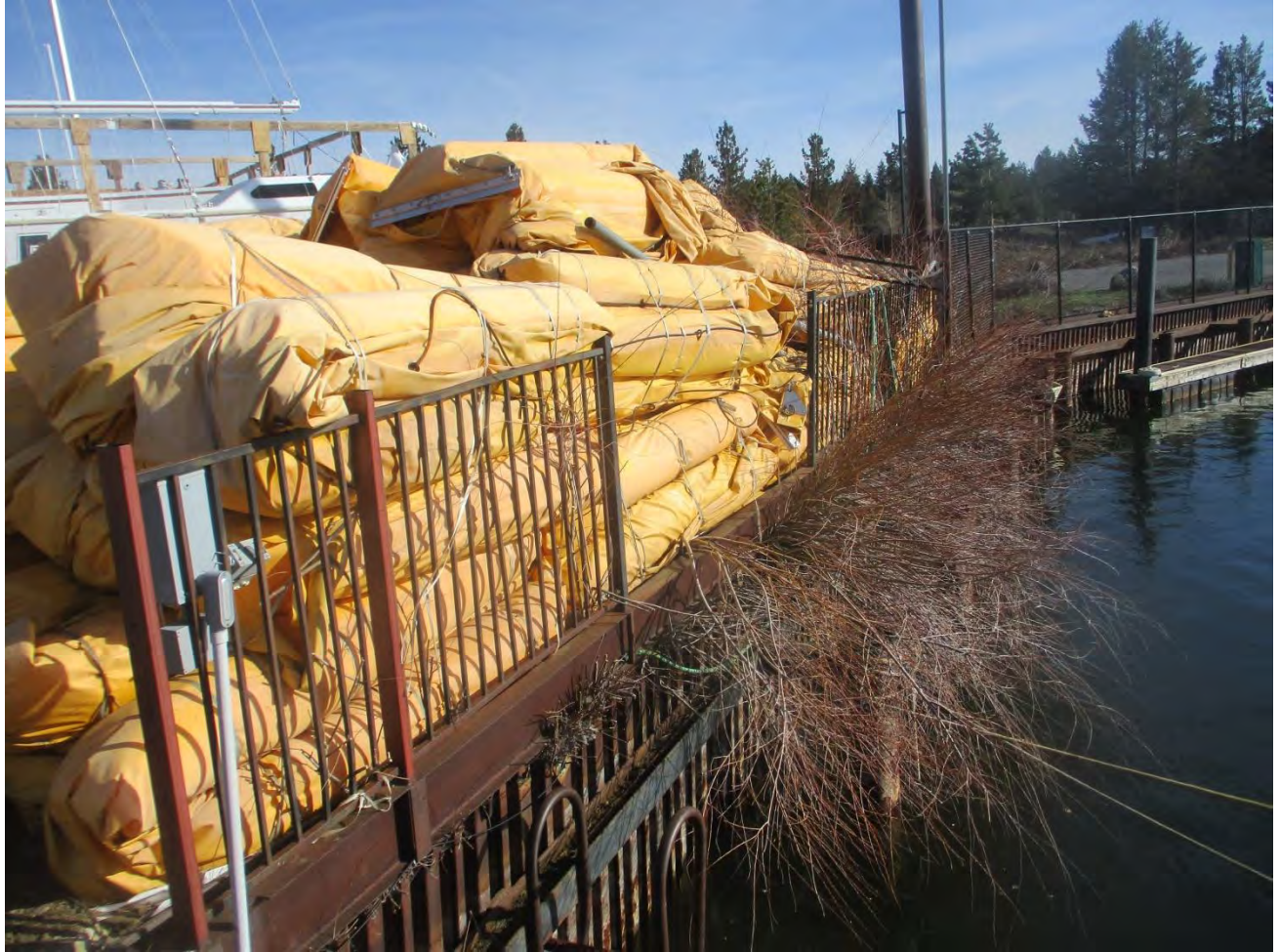
Turbidity curtain, plastic, stored adjacent to waters. Presumably ready for deployment, but covered in a coating of fine white microplastic dust from weathering and/or UV light exposure. (8071)
