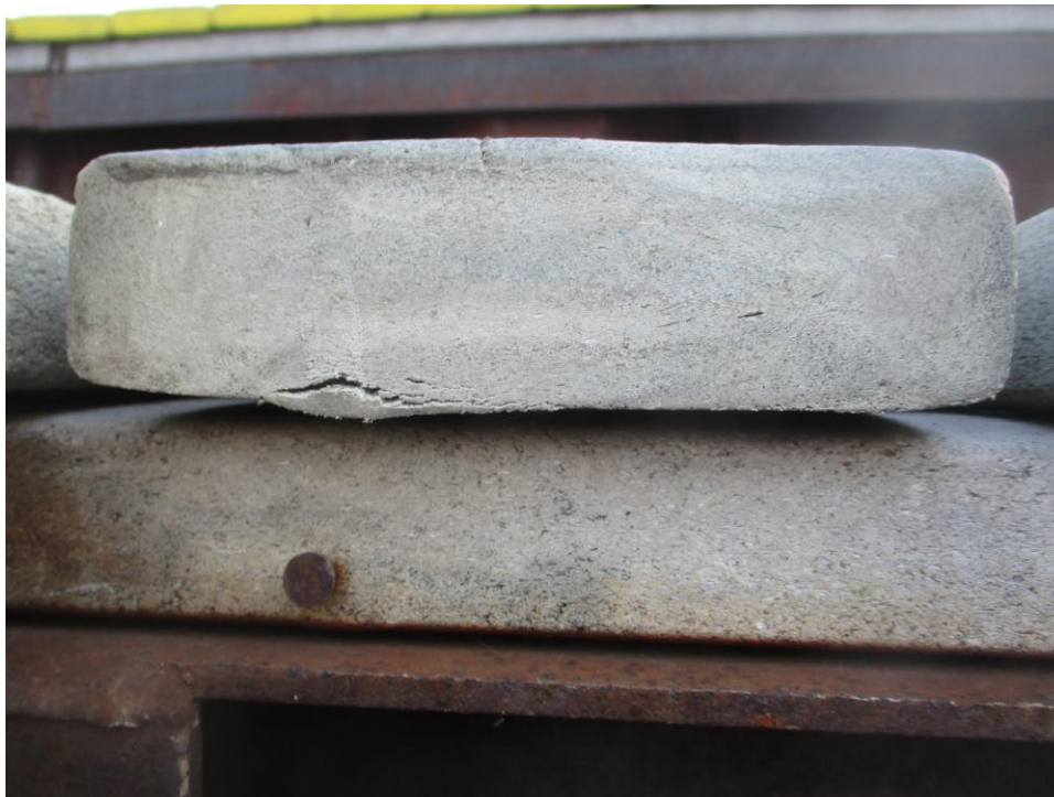
End-view of plastic deck boards showing cracking. (5430)
