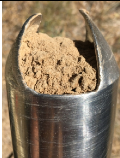
Photo 11A. Soil matrix at 31 in. with 5% Fe redox features
