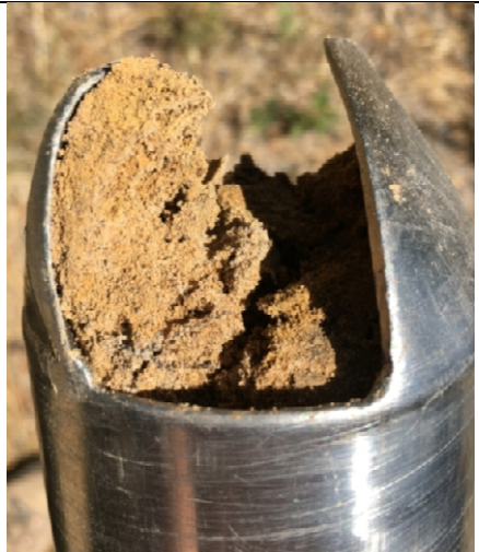
Photo 11C. Soil matrix at 54 in. with 20% Fe redox features.
