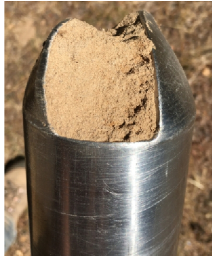
Photo 6A. Soil matrix at 32 in. with 1% Fe redox features.
