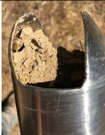
Photo 6B. Soil matrix at 37 in. with 5 to 10% Fe redox features.
