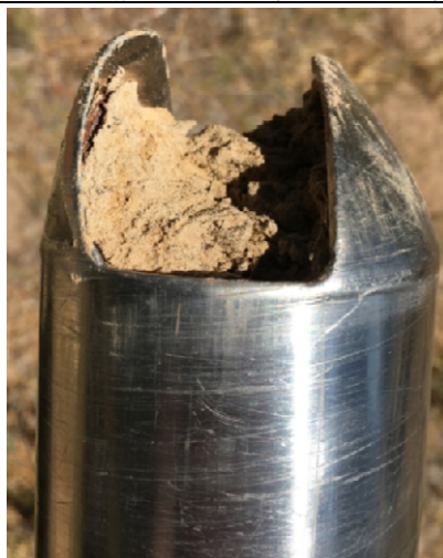
Photo 11B. Soil matrix at 41 in. with 10 to 15% Fe redox features.
