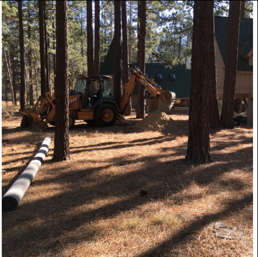
Photo 2. View east at vicinity of Soil Pit 1. 2% slope and E x SE aspect. Lake terrace landform composed of granitic outwash.
