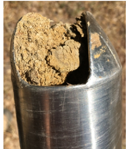
Photo 6C. Soil matrix at 52 in. with 10 to 15% Fe redox features
