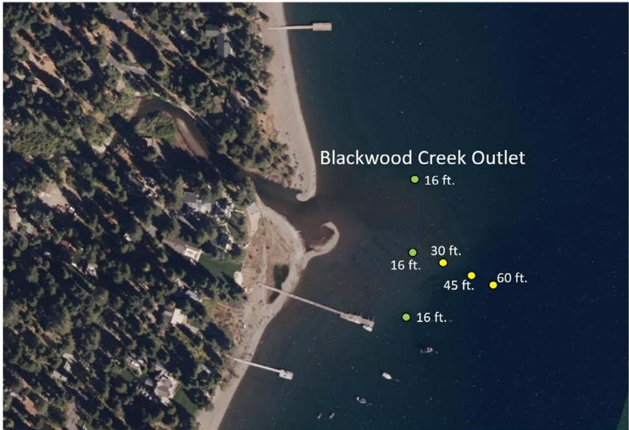
Figure 4. Map of proposed subsurface sensor locations at the outlet of Blackwood Creek on the west shore of Lake Tahoe. Subsurface buoy locations are approximated on the map as yellow circles at 30, 45, 60 ft. of water depth aligned with the creek outlet. The 16 ft depth cinderblock deployments are green circles because they will not be buoys. We have access to this area through public beach access off of Tallac Ave.
