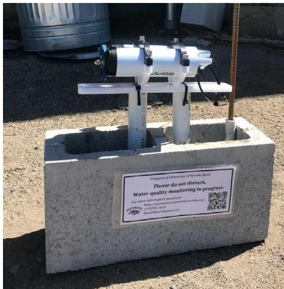
Figure 1. Example of sensor cinderblock deployment design for nearshore locations.. This design is only appropriate for the closest locations where the sensor can be assumed to capture most of the water column. Oxygen and water temperature sensors are in white and have automated wipers attached to ensure minimal biofouling during two-month deployments.
