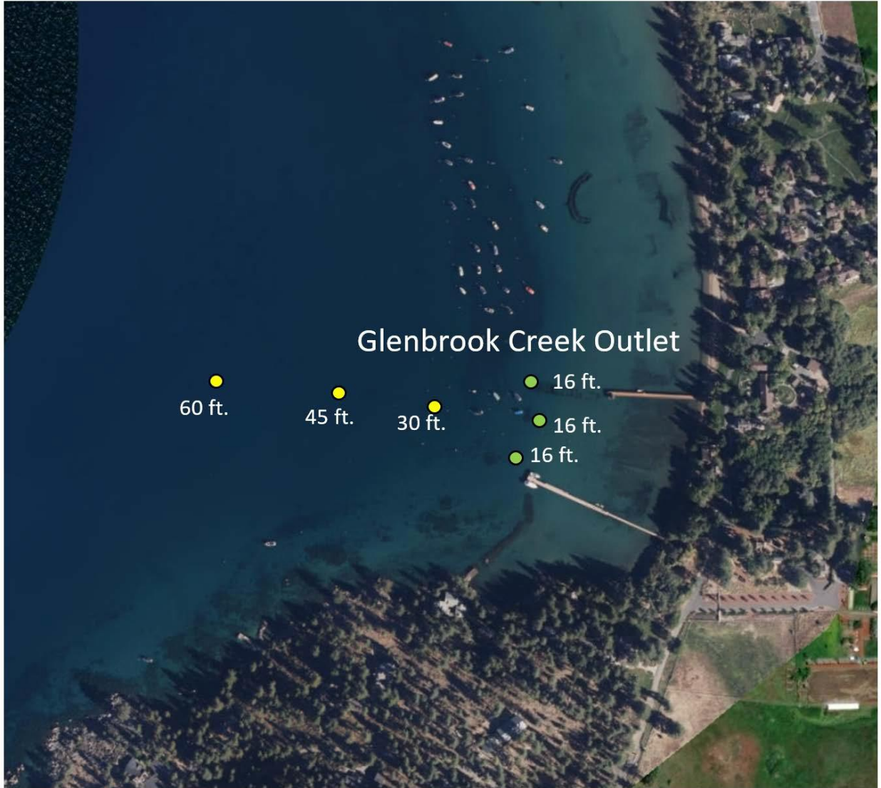
Figure 3. Map of proposed subsurface sensor locations at the outlet of Glenbrook Creek on the east shore of Lake Tahoe. Subsurface buoy locations are approximated on the map as yellow circles at 30, 45, 60 ft. of water depth aligned with the creek outlet. The 16 ft depth cinderblock deployments are green circles because they will not be buoys. We have access to this area through Sudeep Chandra's connections with property owners in the community.
