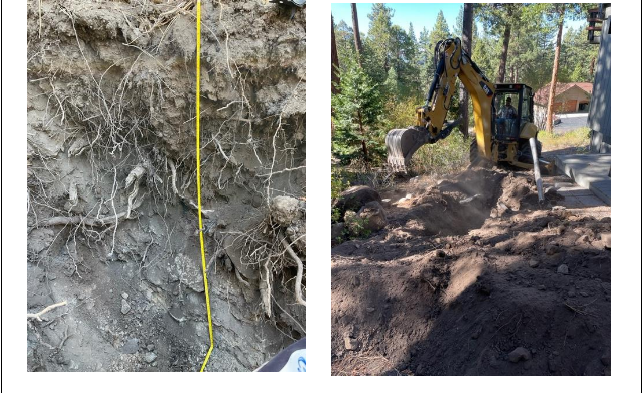
Photo 1 – a. Pit to a depth of 65 inches. Photo 1- b. View looking from above pit towards the west, along the south side of the residence.
