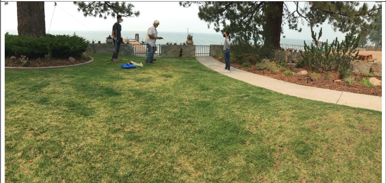
Photo 2 – View westward toward Stop 2 location (west of residence), where a hole was hand-augered to 60 inches. The profile showed no significant soil development aside from an A horizon. The soil is excessively drained due to underlying sand layers and lacks any indication of seasonal high water table. Several large Jeffrey pine trees attest this has been a stabilized barrier beach ridge for a century or more.
