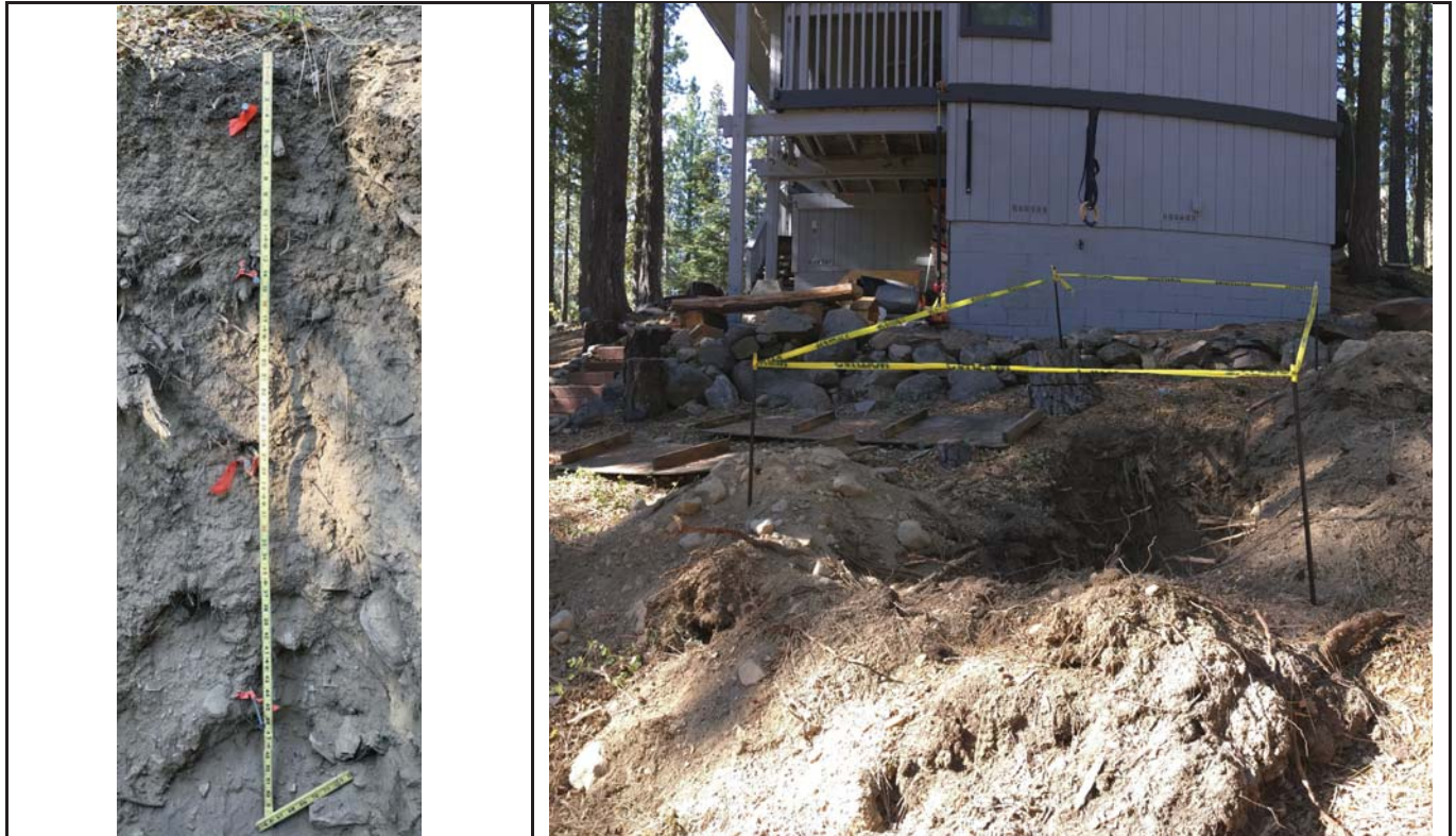
Photo A – View of soil profile showing bottom depth of 55 inches. Root penetration to bottom and no indication of seasonal water table.
