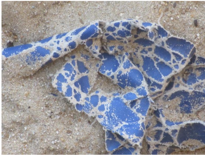
Discarded plastic shard from turbidity curtain in use, plastic deteriorating. (4241)
