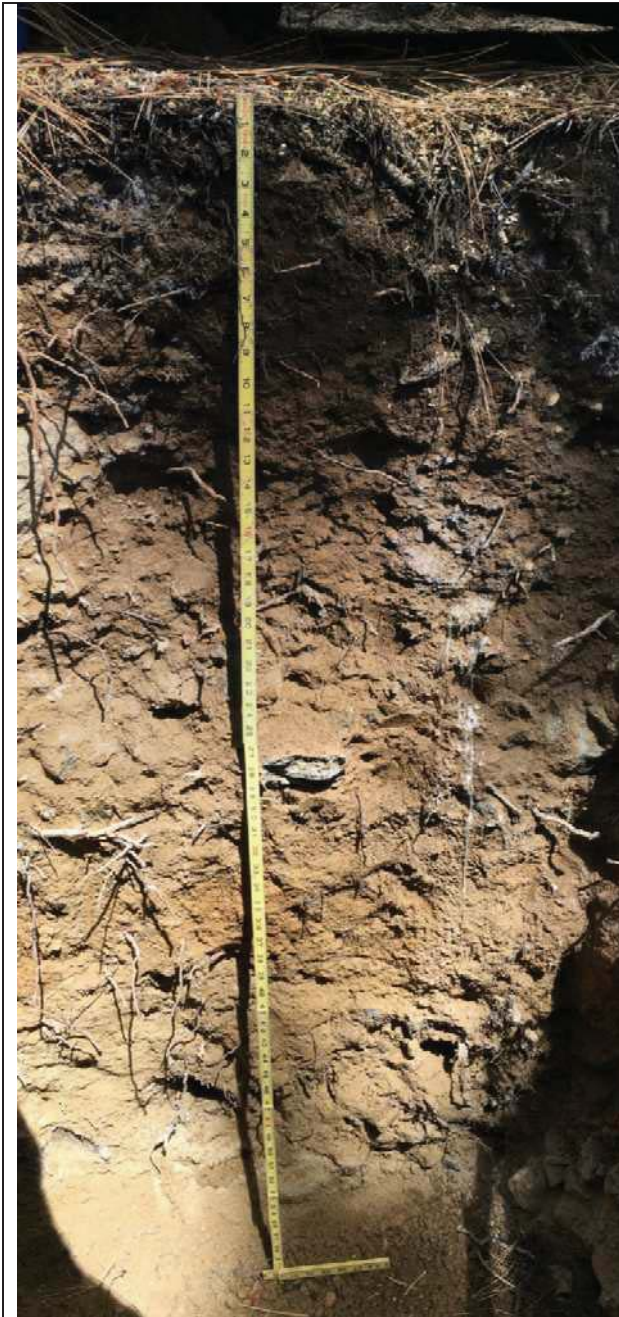
Photo 5 – Soil profile in soil pit located northwest of the residence. The topsoil layer is 24 inches thick and composed of eroded soil from hillside above (colluvium). The subsoil below is 30 inches thick and has thin clay films that qualify those layers as argillic (slightly lower permeability) Profile lacks root-restricting layer (such as a high water table or brittle layer), so this unnamed soil (XXX) qualifies as Class 4, as per Table 4 of the Bailey land capability report.
