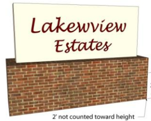
Figure 38.7.3-B: Additional Height for Freestanding Signs
