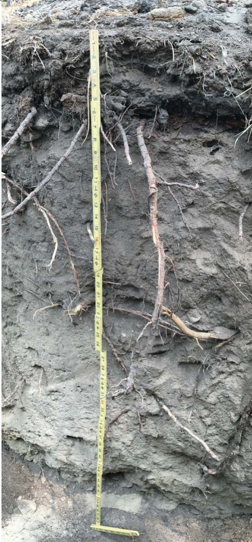
Photo 5 – Soil profile for lower terrace (Stop 1). Topsoil layer is 28 in thick and composed of loamy sand likely deposited as a dune, as apparent by the lack of gravels. Underlying parent material is 32+ inches thick and lacks in-situ soil development. Profile lacks root-restricting layer (such as a seasonal high water table or dense fragipan). While similar to Gefo series, this unnamed soil (XXX, Class 6) has substantially thicker “A” horizon, less gravels, and less soil development than that series. As per Table 4 of Land-Capability Classification of the Lake Tahoe Basin, California-Nevada, A Guide for Planning (Rbt. Bailey, 1974). There is also a small band of Class 4 soil with same conditions, but 16 to 30% slopes.
