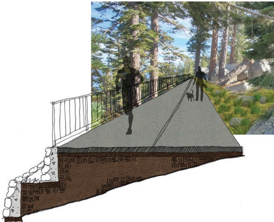
Figure 3.6: Cross section of trail, showcasing terraced slope through forest - potential condition (visualization by I. Avila)
