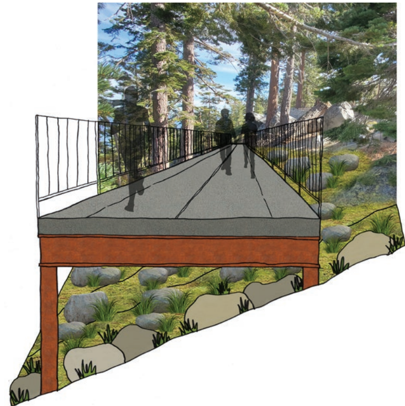
Figure 3.7: Cross section of trail, showcasing a pier-supported trail, which minimizes scenic impacts and ground disturbance (visualization by I. Avila)
