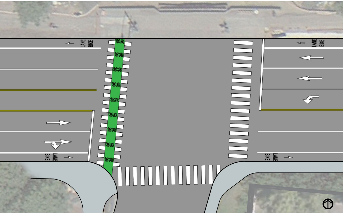
Recommended Rufus Allen/US 50 intersection enhancements
