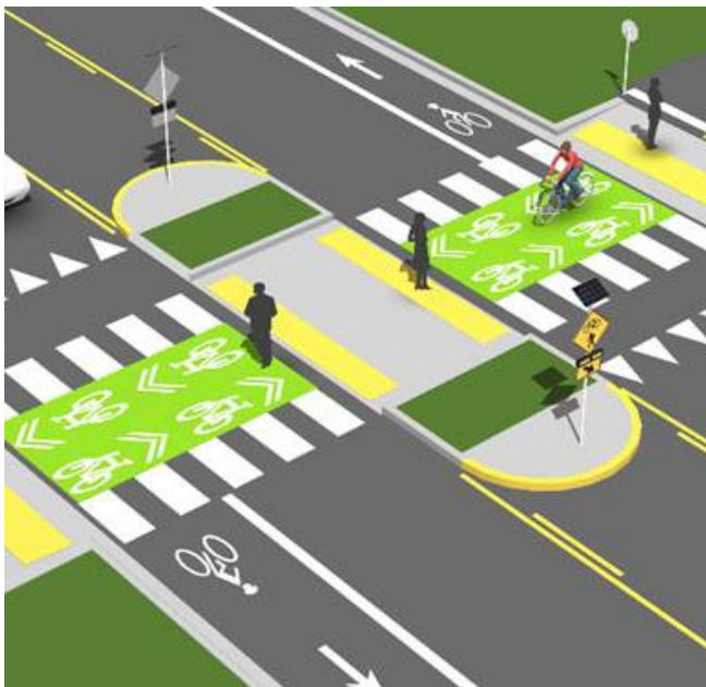
Crossbike example: bike crossing lanes adjacent to the pedestrian crosswalk
