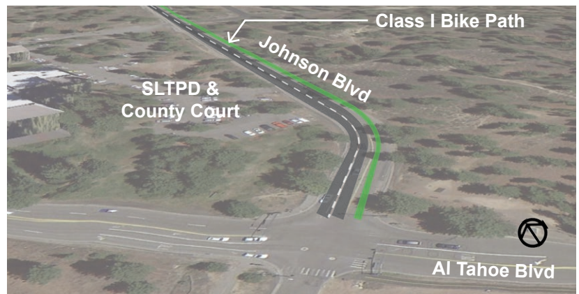
Aerial diagram of Johnson Boulevard Alternative 1 mobility improvements: Class I bike path and narrowed travel lanes
