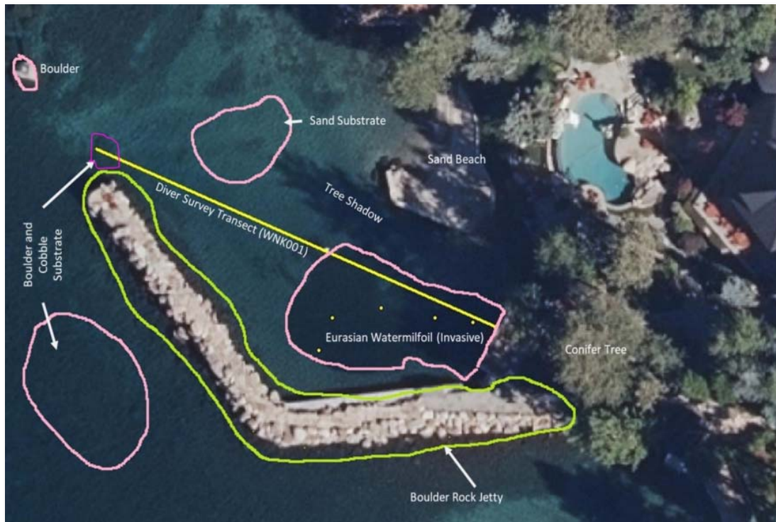
An example of LiDAR and high-resolution imagery used to show lake bottom features and to identify aquatic invasive species.
