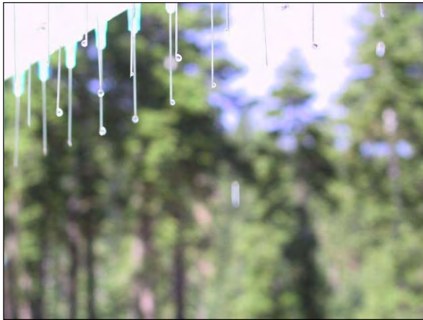
Figure 7. Rain drops are generated from more than 800 hypodermic needles on the rainfall simulator.
