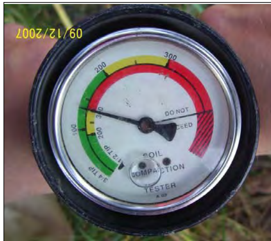
Figure 11. Cone penetrometer dial, showing pressure applied in pounds per square inch.
