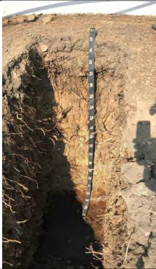
Photo 3 – Soil profile for supplemental soil pit located on south side of hotel. This soil is similar to 11/19/19-1 and best resembles the Jorge-Tahoma soils in the 1974 soil survey.
