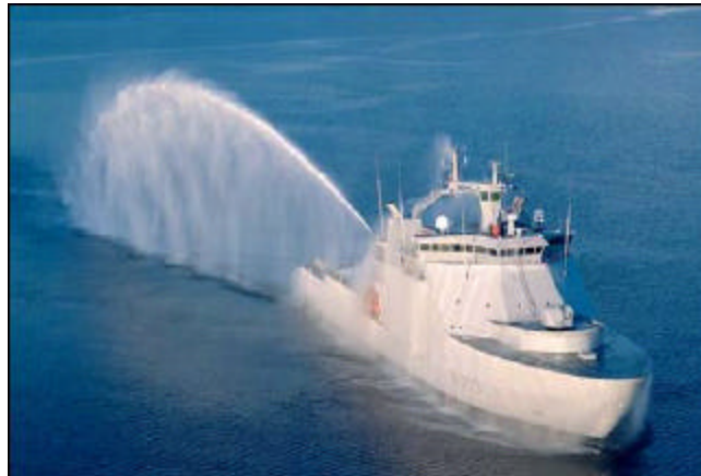
Fig. 2.6: “K/V Svalbard”, Ice breaking coast guard vessel with podded propulsion for the Norwegian Navy.
