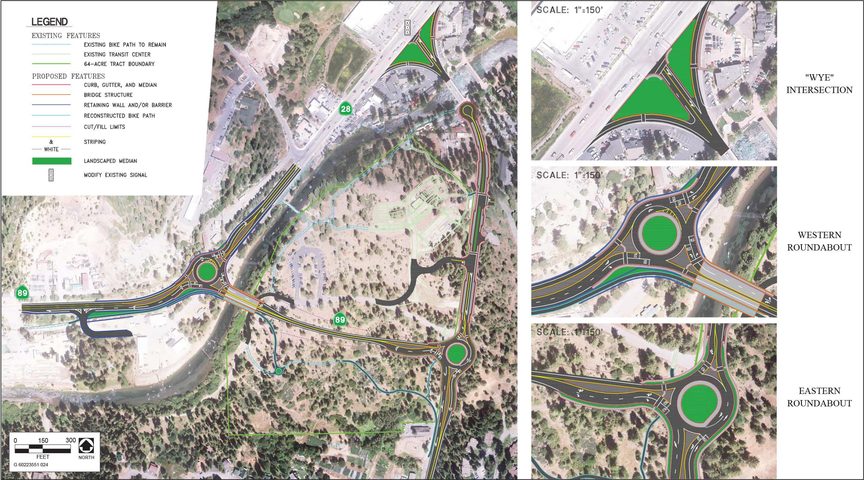
Figure 1-5: Alternative 2 — New Alignment, Close Existing SR 89 to Vehicle Traffic
