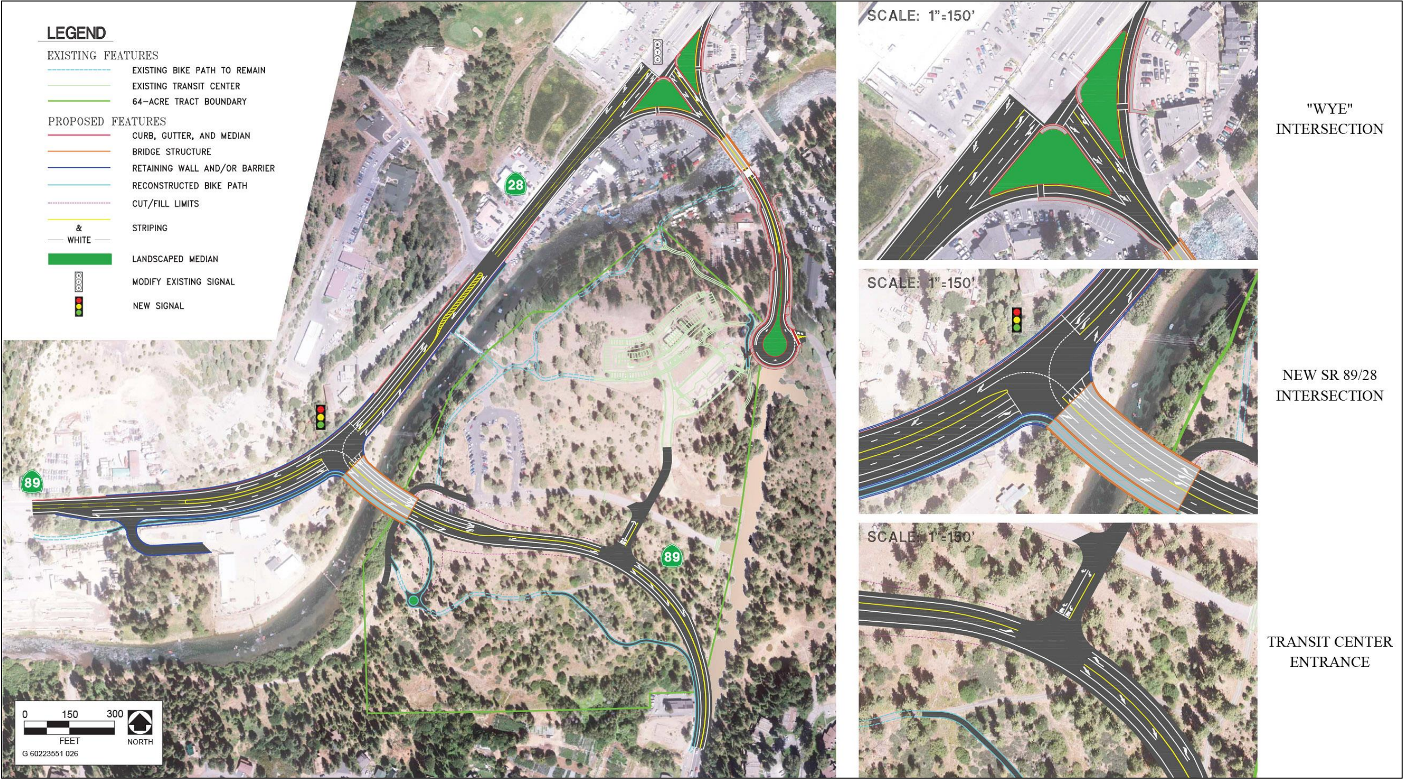
Figure 1-7: Alternative 4 — New Alignment, No Roundabouts, Existing SR 89 Becomes a Cul-de-sac on the South Side of the Bridge
