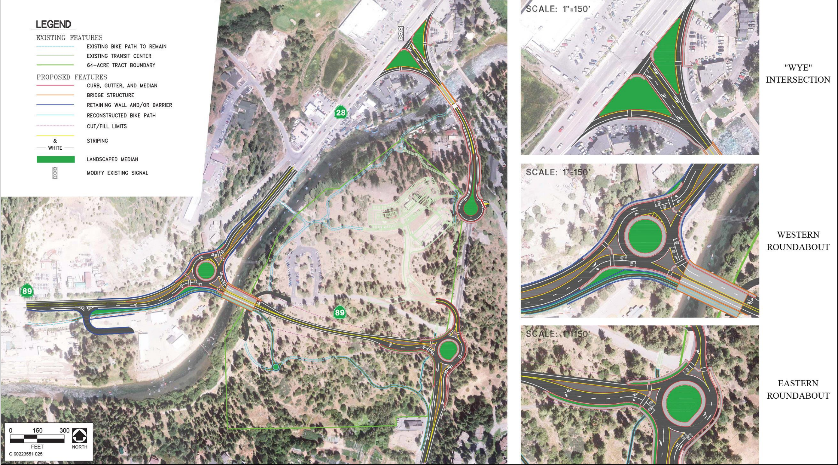
Figure 1-6: Alternative 3 — New Alignment, Existing SR 89 Becomes a Cul-de-sac on the South Side of the Bridge
