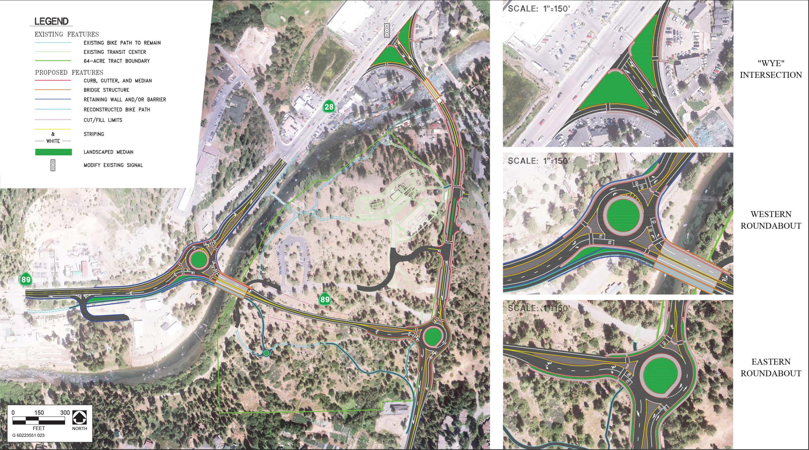
Figure 1-4: Alternative 1 — New Alignment, Existing SR 89 Open to Local Traffic Only
