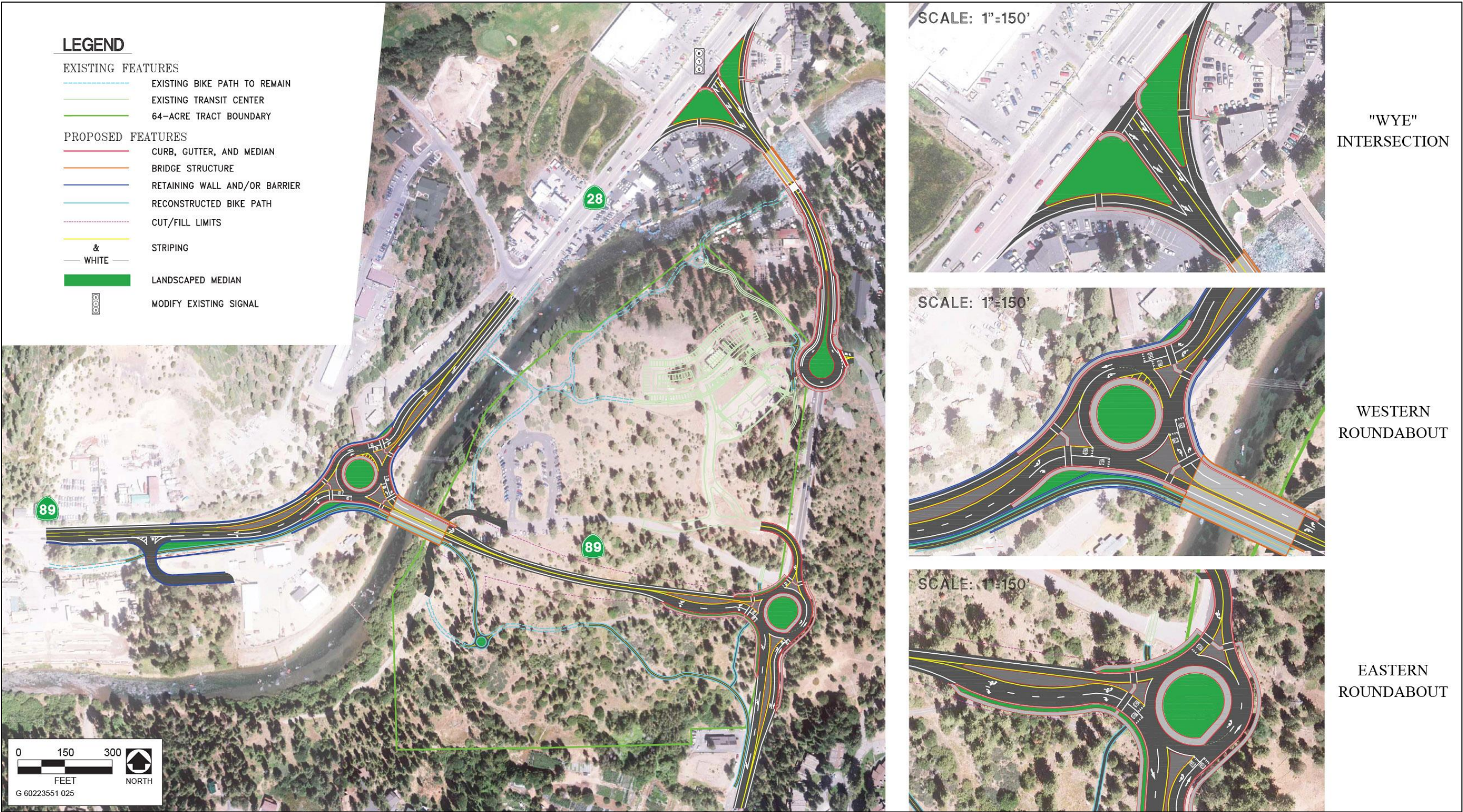
Figure 2-6: Alternative 3—New Alignment – Existing SR 89 Becomes a Cul-de-sac on the South Side of the Bridge
