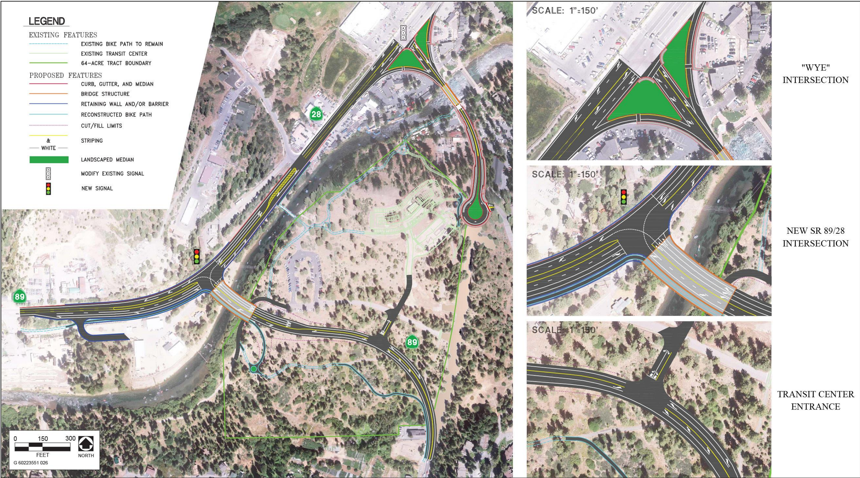
Figure 2-7: Alternative 4—New Alignment, No Roundabouts – Existing SR 89 Becomes a Cul-de-sac on the South Side of the Bridge
