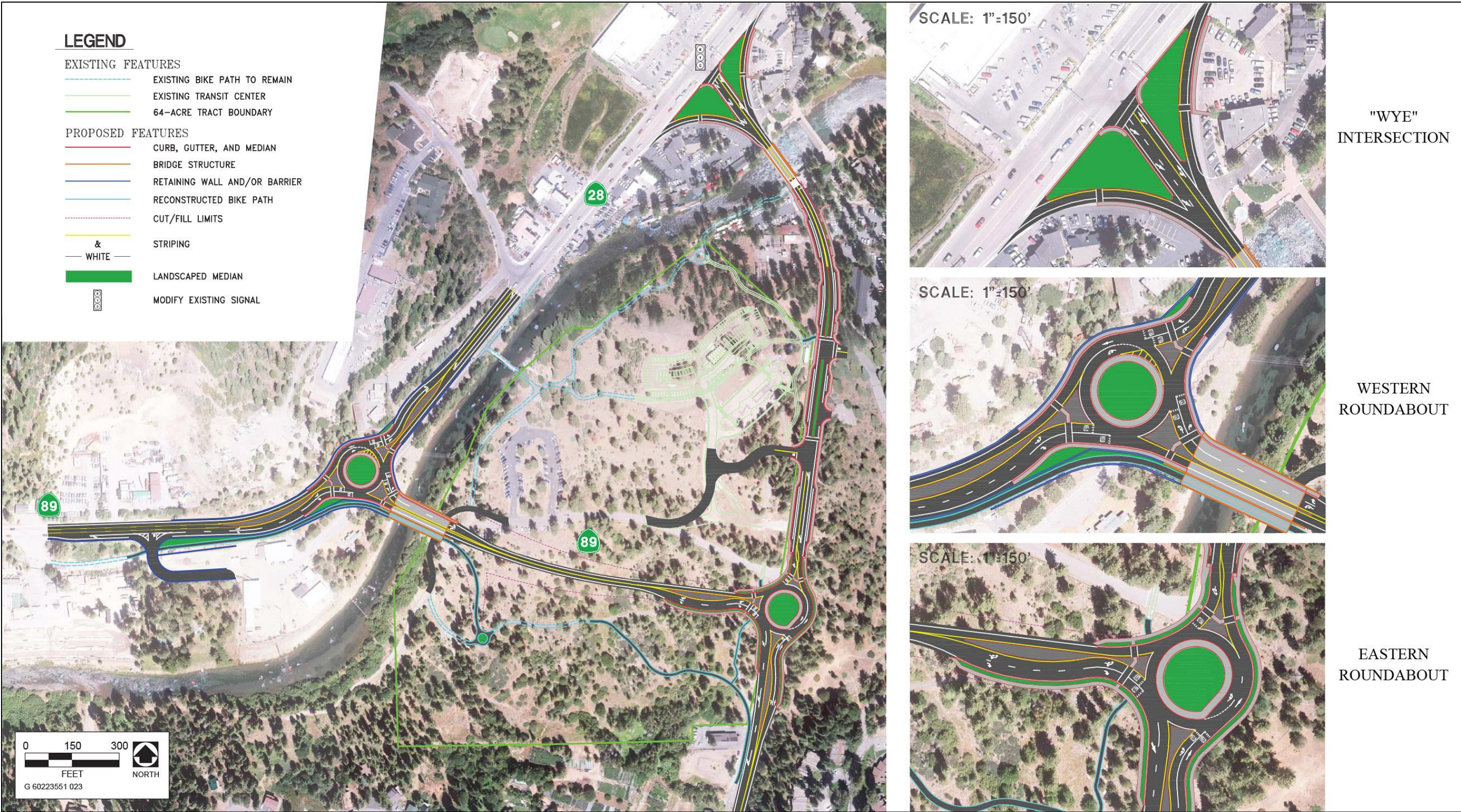
Figure 2-4: Alternative 1—New Alignment – Existing SR 89 Open to Local Traffic Only
