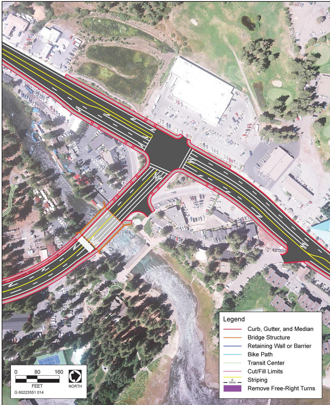
Figure 2-8: Alternative 6— Replace and Widen Existing Bridge, Modify Lane Geometrics at Existing Wye Intersection
