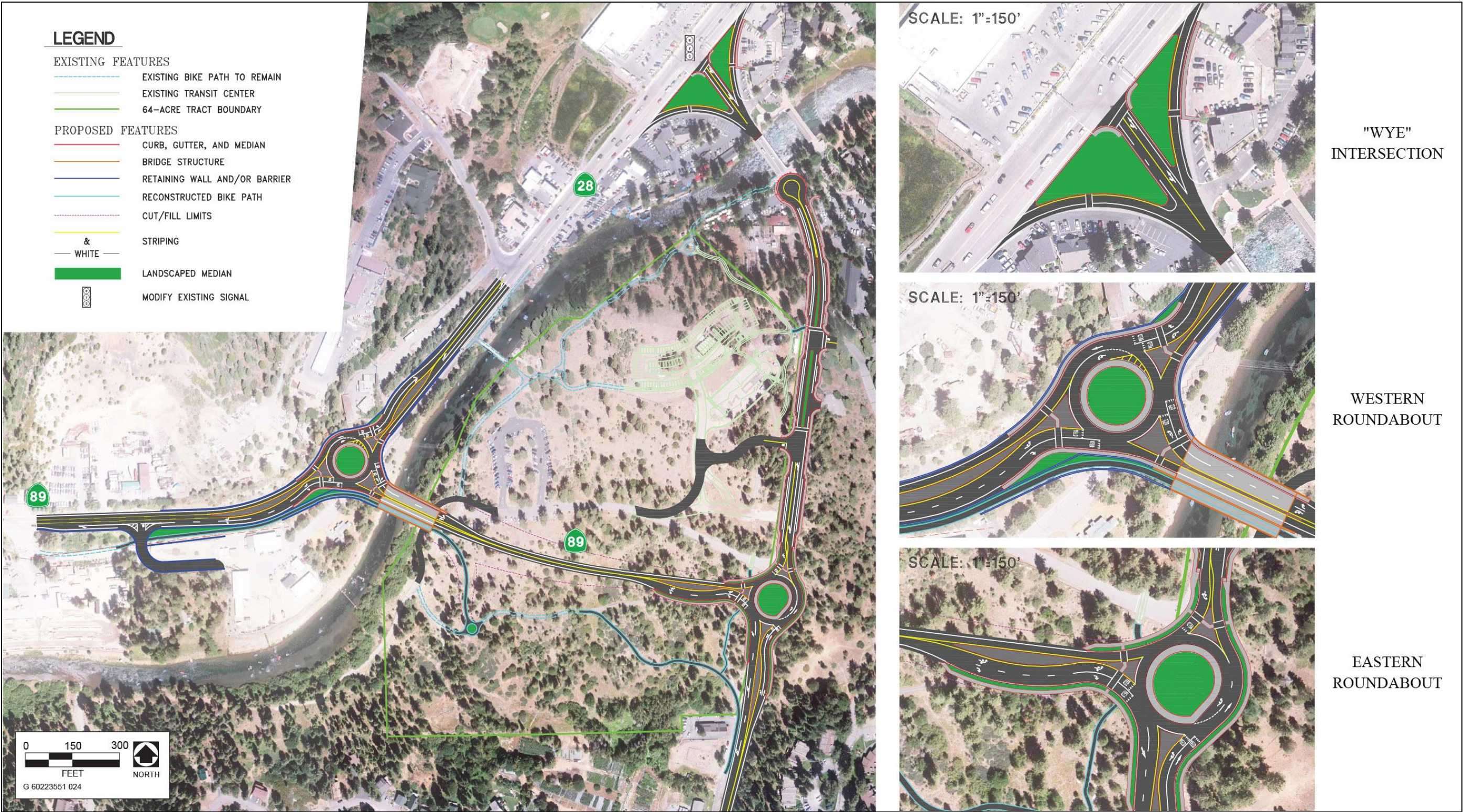
Figure 2-5: Alternative 2—New Alignment – Close Existing SR 89 to Vehicle Traffic
