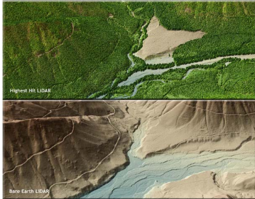
Caption: LiDAR data collected in Lewis County, Washington for the Puget Sound LiDAR Consortium showing "highest hit" and "bare earth" data. This data will provide agencies with a similar capability of measuring terrain characteristics of the Lake Tahoe Basin. Image provided by Watershed Science, Inc.
