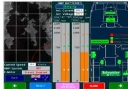
Figure 2: Easy to use interface on the Magelis HMI allows the ferry pilot real-time access to the propulsion system
