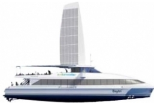
Figure 1: Solar Sailor's patented 'solarsail' technology harnesses renewable solar and wind energies to create energy efficient ferries
