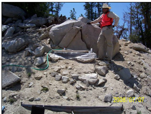
Figure 9. The runoff simulator at the Skyline trail. The PVC pipe is visible just below the boulder and the collection frame is at the bottom of the photo.
