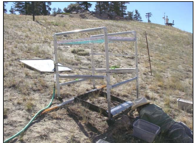
Figure 8. Rainfall simulation in action at the Gunbarrel Top Terminal Slope monitoring area.
