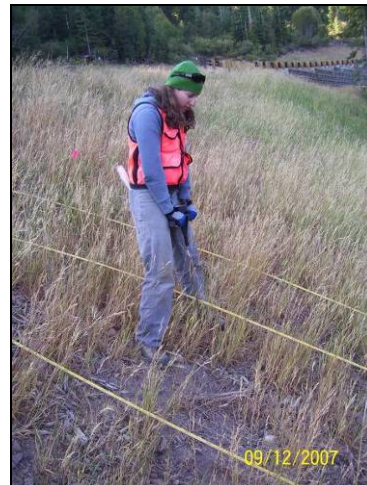
Figure 12. Conducting cone penetrometer readings along transects.
