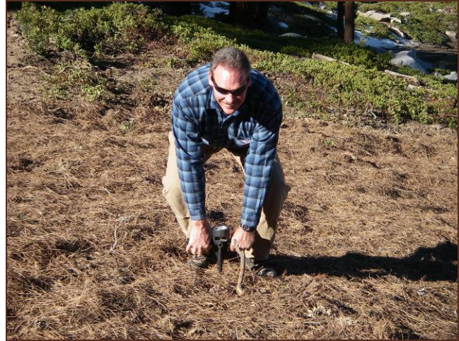
Figure 168. Jim Larmore checks tilling depth with a cone penetrometer.
