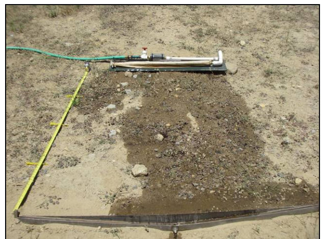
Figure 10. The runoff simulator and test area post-simulation at the Lakeview Lodge Patsy's Trail monitoring site. The PVC pipe is visible at the top of the photo and the collection frame is at the bottom.
