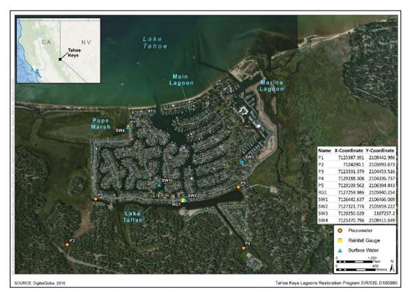
Figure 1. Locations and coordinates for piezometers, surface water level recorders, and a rain gauge at Tahoe Keys.
