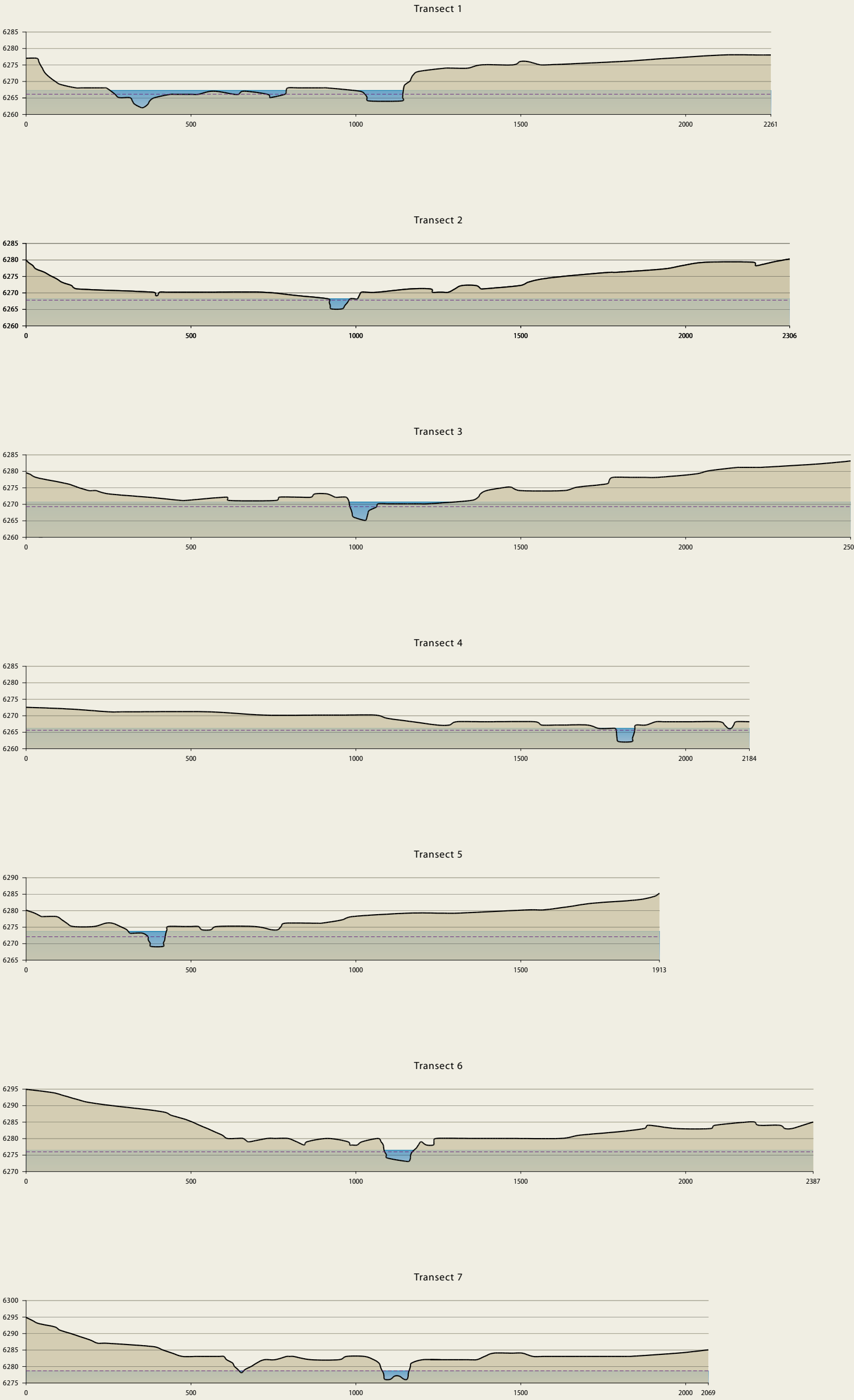
Figure 21: Upper Truckee Transects, 550cfs Estimated changes in water surface elevation, plotted on valley sections (Figure 20).
